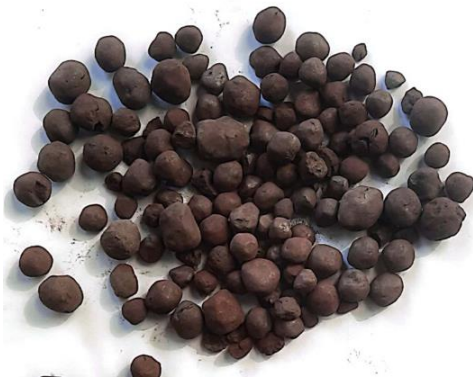
Fig. 1. Iron pellets and powder used in the mixing design
