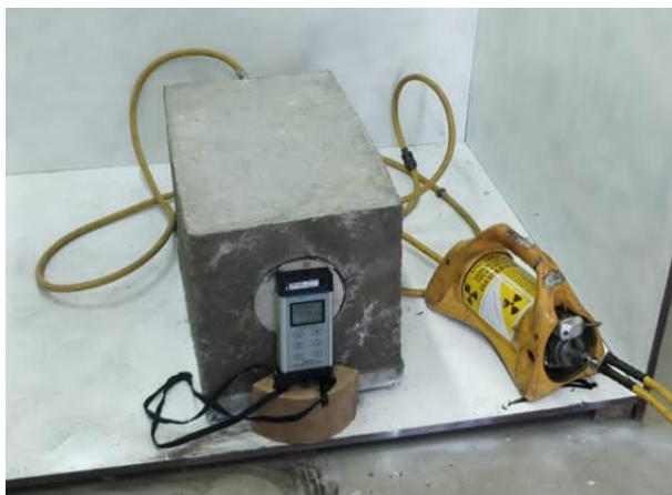
Fig. 2. Gamma source, detector, and the condition of the specimen
