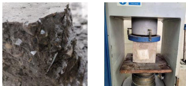
Fig. 4. Compressive strength fracture test of the cubic specimen with concrete breaker jack, Broken specimen of self-compacting concrete with fiber and iron oxide.
