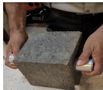
Fig. 3. Testing the ultrasonic pulse speed on the test piece.
