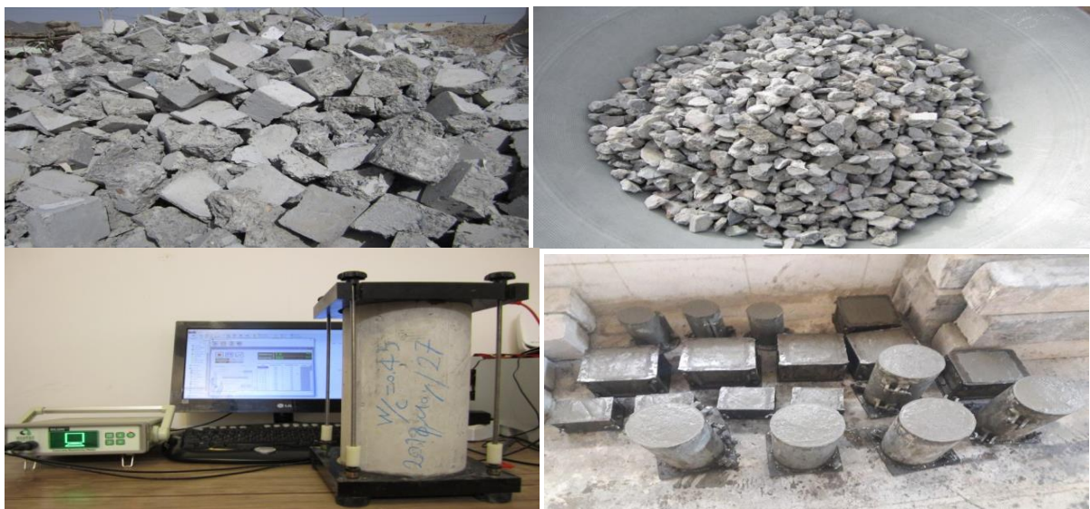
Fig. 1. Construction and testing electrical resistance of specimens
