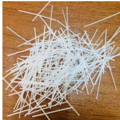
Fig. 1. Fibers used in the study, (a) Polypropylene (b) Barchip 48 (c) Forta-ferro.
