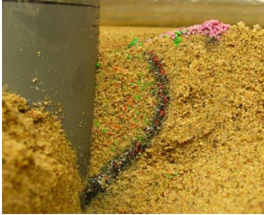
Fig. 1. Convective movement of sand particles around the pile [9].
