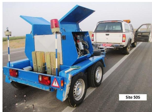
Fig. 1. FWD testing on a site
