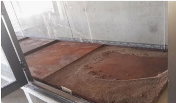
Fig. 1. Wind erosion test of primary soil samples
