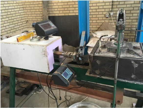
Fig. 1. Geotextile pull-out device
