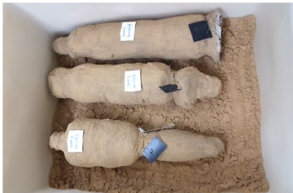
Fig. 2. Columns inserted in the box for curing
