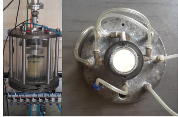
Figure 1. Unsaturated triaxial chamber and ceramic disk on bottom pedestal
