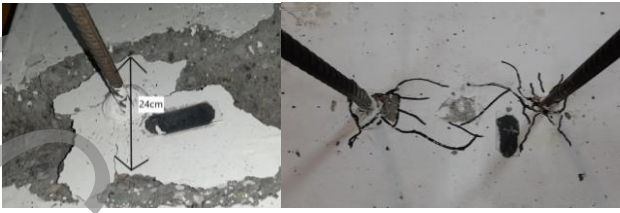
a. Single test b. Group test Figure 1. Example of tension test results
