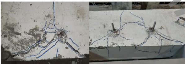
a. Single test b. Group test Figure 2. Example of shear test results
