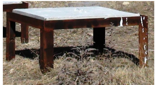
Figure 1. The setup of blast loading test and arrangement of support frame.
