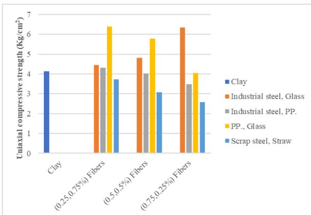
Fig. 6: Diagram of uniaxial compressive strength of soil combined with five kind of fibers and with different percentages as a pairs compound
