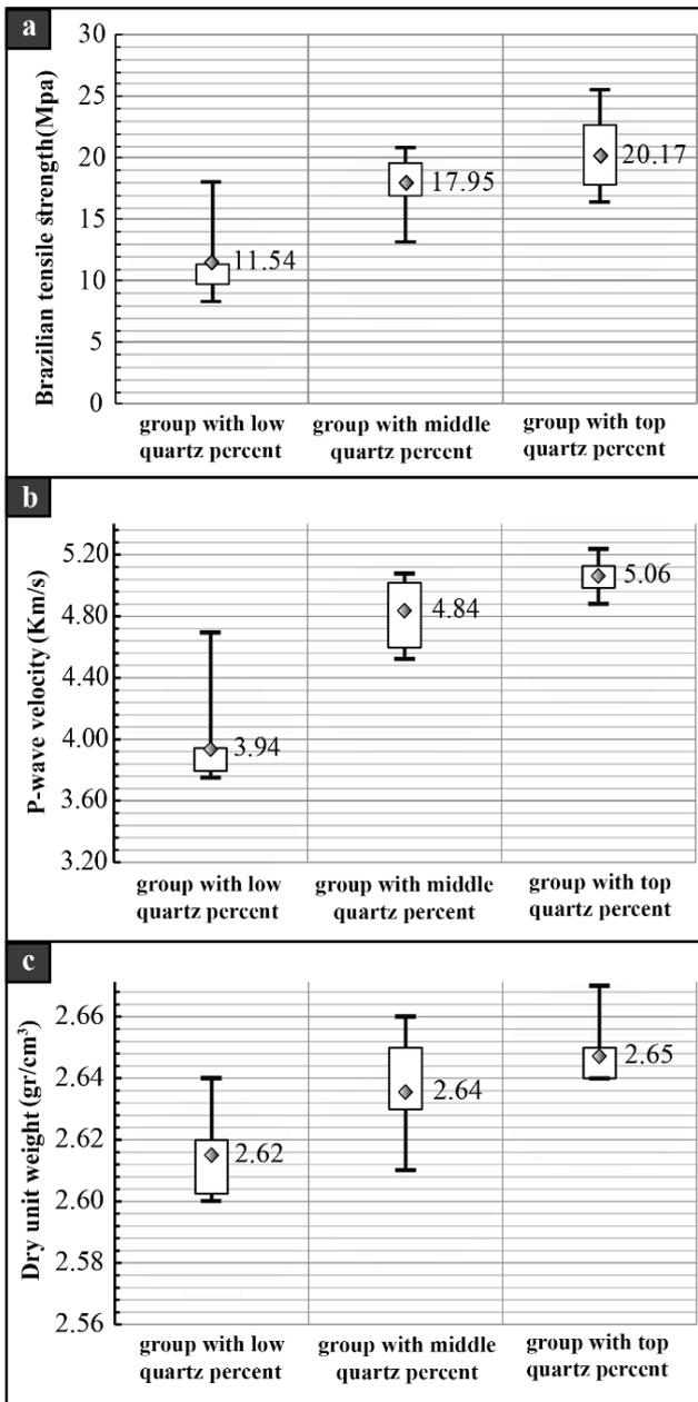
**Fig. 1. Graphs related to changes in the studied engineering properties of the sandstone in relation to the quartz mineral content (a) Brazilian tensile strength (B) p-wave velocity (c) dry unit weight**
