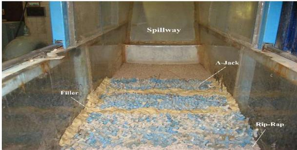
**Fig 1. The protected bed with SLC and rip-rap materials****Table 2. Cost of the Rip-Rap and SLCE in an area of 100 m<sup>2</sup>**
