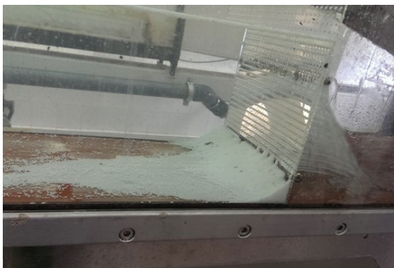
Fig. 4. The accumulation of sedimentary materials upstream the obstacle
