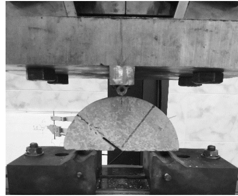
Fig. 4. SCB test set-up
