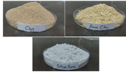
Fig. 3. Additional materials to the movable bed of downstream of stepped spillway
