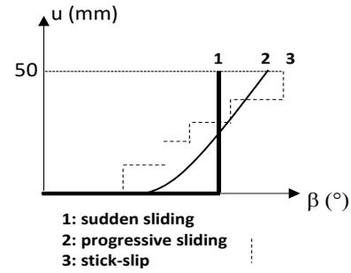
Fig. 3. Different mechanisms of sliding upper box [4].
