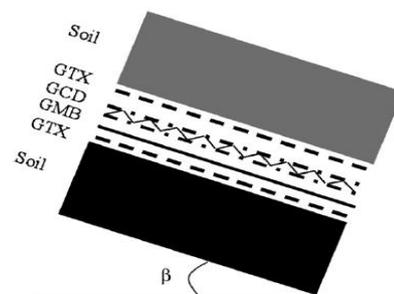
Fig. 1. Typical liner system on slope [4].
