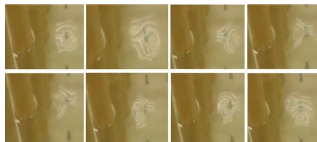
Fig. 1. A sample of vortex shedding from obstacles in the laboratory flume of present study
