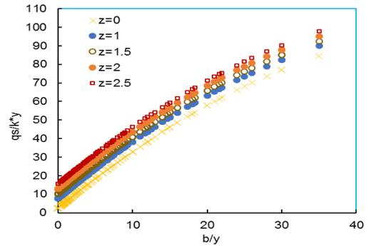
Fig. 8. Relationship between  $b/y$  and  $q_s/K_y$  in different values for  $z$
