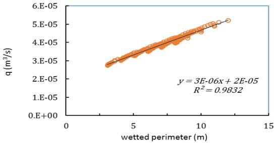
Fig. 6. The effect of the wetted perimeter on the seepage discharge in different trapezoidal, rectangular and triangular sections
