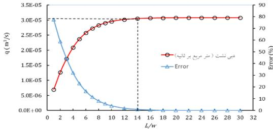
Fig. 5. The seepage and error changes relative to the L/W in the trapezoidal section.
