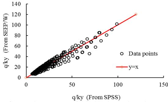
Fig. 7. Comparison between SEEP/W simulation with regression (Equation 5) using SPSS software
