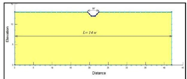
Fig. 4. Trapezoidal channel and recommended lateral distance .for determining boundary condition
