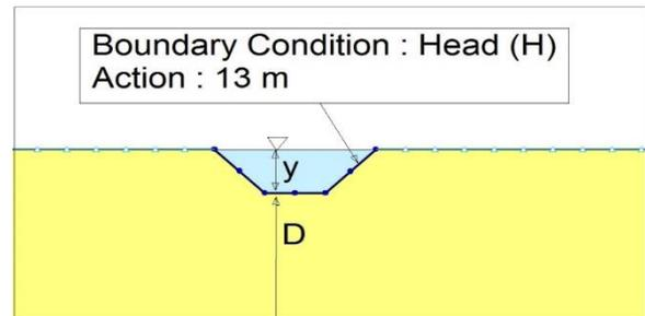
Fig. 2. Boundary condition for the bottom and side walls of the trapezoidal cross section
