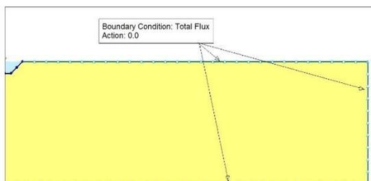
Fig. 3. Impermeable boundary conditions for the bed and walls of the trapezoidal earth channel model (half of the channel is seen on the left).
