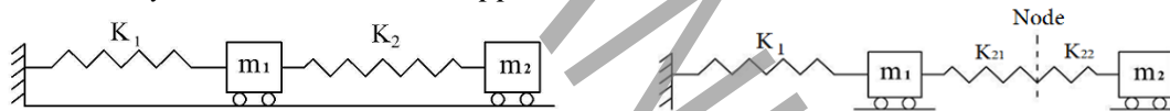
Fig.2: A 2-DOF stable system which has a support (left), assuming node location and dividing the primary spring into K 21 and K 22 (right)
