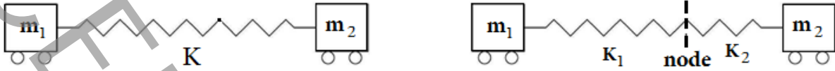
Fig.1: Dividing the primary spring (left) into two adjust series springs ( K_1 & K_2 ) from the node location (right)
