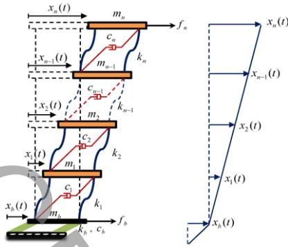
**Figure 1. Shear model of  $n$  degree freedom structure equipped with base isolation.**
