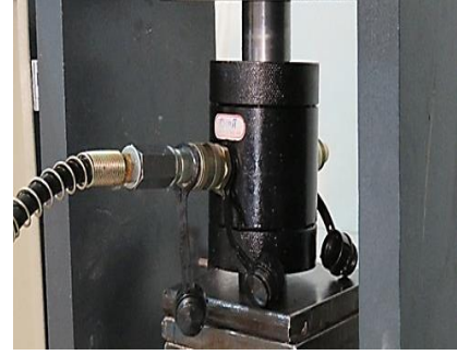
Figure 1. A Hoek cell for triaxial test.
