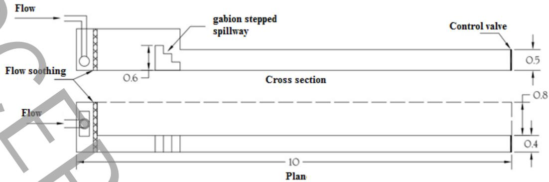
Figure 1: View of the laboratory flow and location of the stepped gabion spillway (dimensions in meters)
