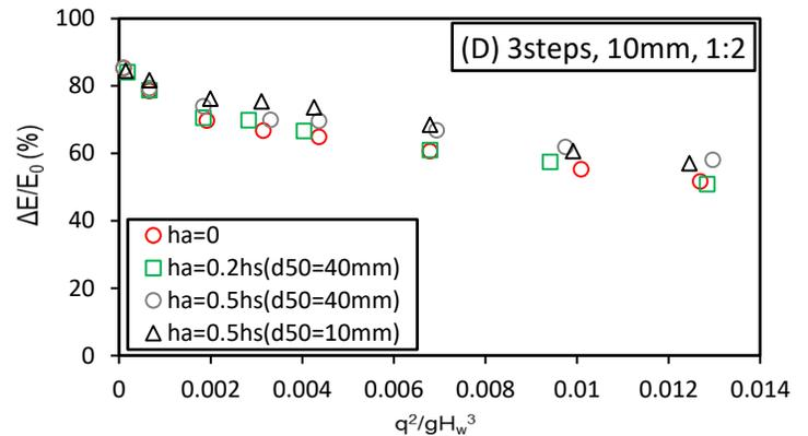
Figure 3: Relative energy loss changes against to  $q^2/gH_w^3$  for gabion rectangular and sloped end sills
