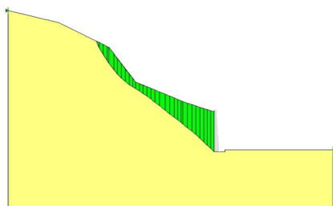
Figure 2 (a). Soil slope status after precipitation without drainage system
