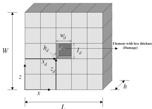
Figure 1. Finite element view of damaged plate
