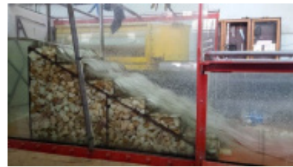
Figure 2. Transitional flow in a weir with 6 steps and slope of 1:2, Q=44 lit/s, d 50 =40 mm
