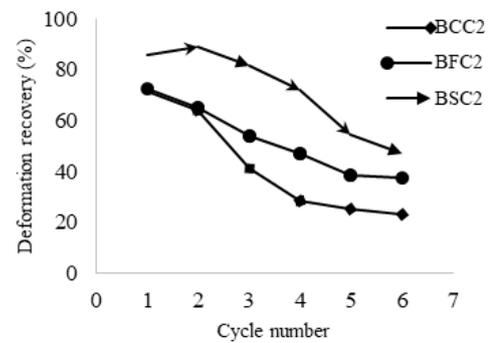
**Figure 3. The ability of deformation recovery for the specimens BCC2, BFC2 and BSC2**
