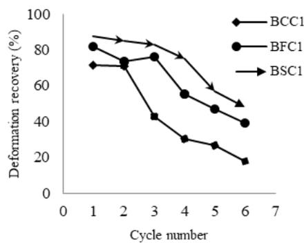
**Figure 2. The ability of deformation recovery for the specimens BCC1, BFC1 and BSC1**
