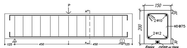
Figure 1. Geometries of beam specimens, reinforcement arrangement and loading configuration
