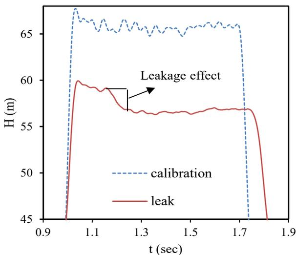
Figure 1. Comparison of Transient Flow Signal Signals in a Healthy Pipeline with Viscoelastic Tubing Leakage
