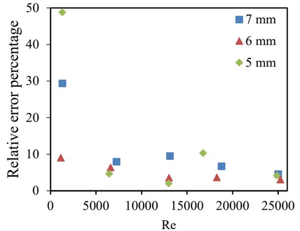
Figure 2. The relative error of computational and laboratory leakage distances in different Reynolds at three leaks of 5, 6 and 7 mm
