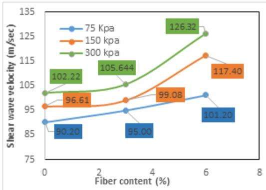
Figure 2. Effect of fiber content and confining stress on shear wave velocity
