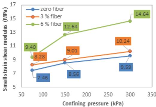
Figure 3. Effect of fiber content and confining stress on small-strain shear modulus
