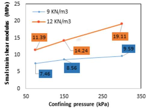
Figure 5. Effect of unit weight on small strain modulus
