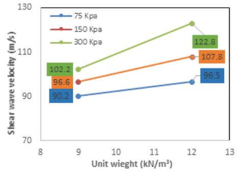
Figure 4. Effect of unit weight on shear wave velocity
