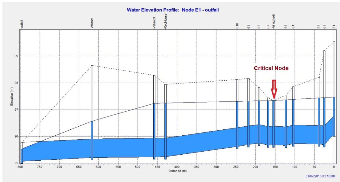
Figure 2. Longitudinal profile of the main conduit and hydraulic line for a 10-year return period
