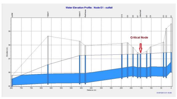
Figure 2. Longitudinal profile of the main conduit and hydraulic line for a 10-year return period
