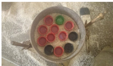
Figure 2: Preparing reinforced sample with layer combination
