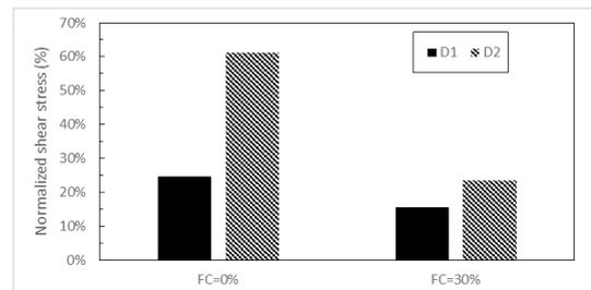
Figure 4.  $\Delta\tau_{EGC} / \tau_{GC}$  for two grain size of aggregate columns
