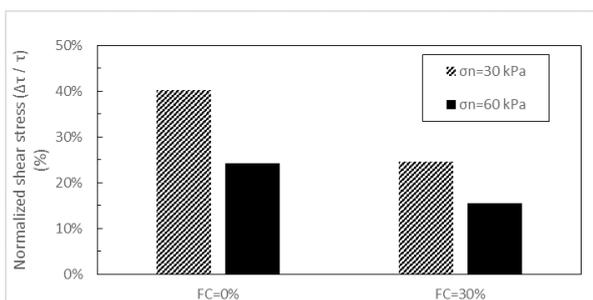
Figure 2. Normalized shear resistance at two normal stress
