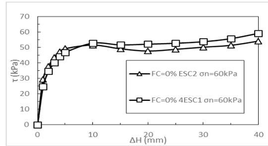
Figure 3. Shear stress vs. displacement of EGCs (FC=0%)
