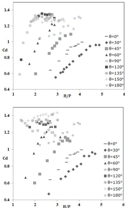
**Figure 3: H/P dimensionless parameter against discharge coefficient, for different angles and diameters, a) Upstream curve and b) Downstream curve**
