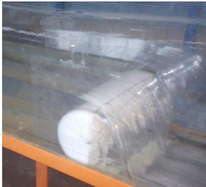
Figure 2: Section of the semi-cylindrical wire-gate in the upstream curve
