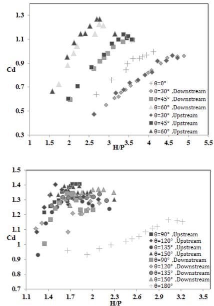
**Figure 4: H/P dimensionless parameter against discharge coefficient, for different angles and diameter of 70 mm**
