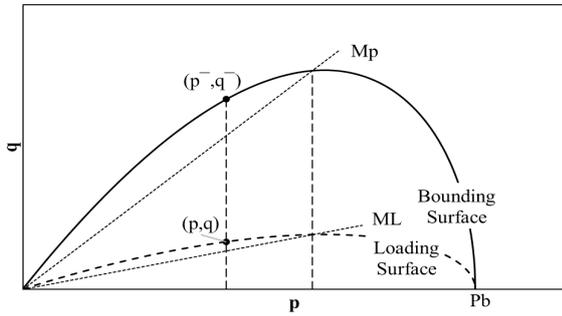
Figure 1. Bounding surface, and determination of loading surface using the mapping rule employed
