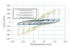
Figure 7: Hysteresis loops for different arrangements of connecting bolts under transverse cyclic loading
