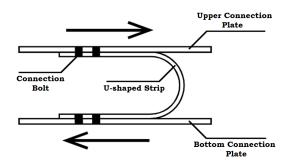
Figure 1: Typical U-shaped damper
