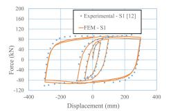
Figure 3: Comparison between simulated and experimental hysteresis loops
