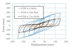
Figure 5: Hysteresis loops with and without simulation of connecting bolts under transverse cyclic loading
