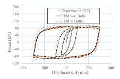
Figure 4: Hysteresis loops with and without simulation of connecting bolts under longitudinal cyclic loading
