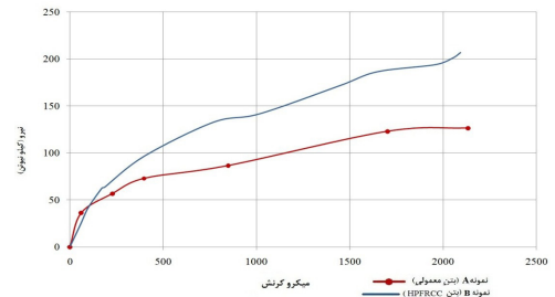
Figure 5. Force-stress curves of diagonal reinforcement specimens A and B
