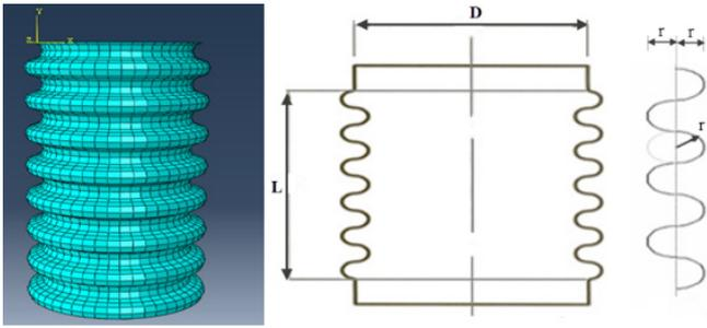
Figure 1. Finite Element model of the specimen
