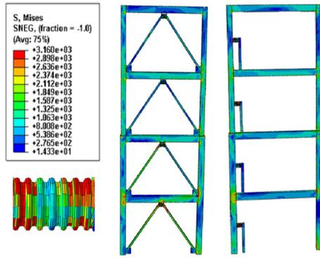
Figure 6. Von-mises stress contour for one story frame with two cases of dampers under a blast with intensity 36 kg/cm<sup>2</sup>
