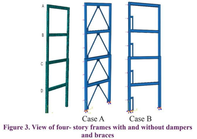
Figure 3. View of four-story frames with and without dampers and braces
