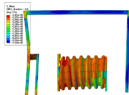
Figure 5. Von-mises stress contour for one story frame with damper case B under a blast with intensity of 36 kg/cm<sup>2</sup>
