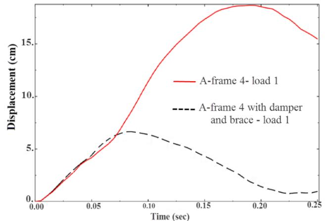
Figure 9. Time history of joint A for a four-story frame with damper cases A and B and without them (blast 36 kg/cm<sup>2</sup>)
