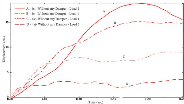
Figure 7. Time history of joint A for a four-story frame with damper cases A and B and without them (under blast of 36 kg/cm<sup>2</sup> intensity)
