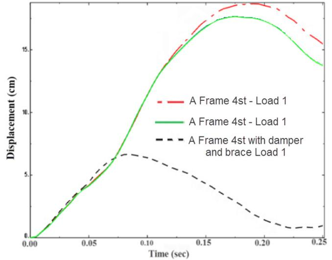
Figure 8. Time history of joint A for a four-story with damper cases A and B and without them (under blast of 36 kg/cm<sup>2</sup> intensity)
