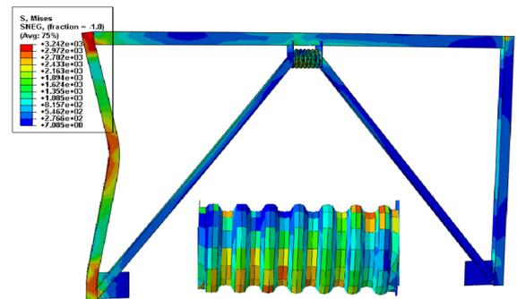
Figure 4. Von-mises stress contour for one story frame with damper case A under a blast with intensity of 36 kg/cm<sup>2</sup>
