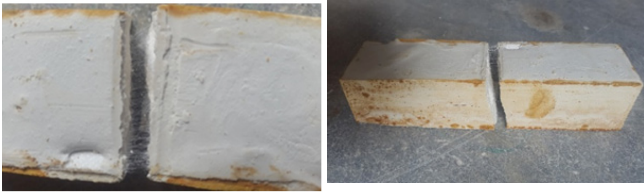
Figure 2. The reinforced samples after the bending test
