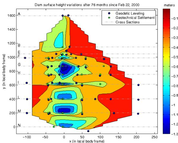
Figure 1. Settlements of the dam surface during 76 months
