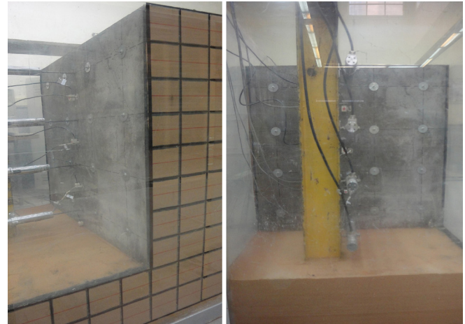
Figure 1. Finished soil-nailed wall model in shaking table box
