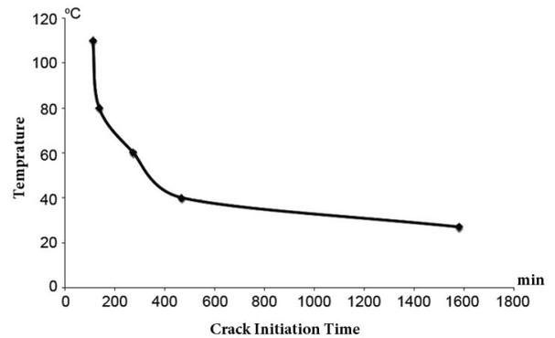
**Figure 2. Effect of temperature on crack initiation time**
