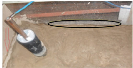
Figure 4. Consolidation of the soil in experiment 2 and voltage of 40 V as a result of draining
