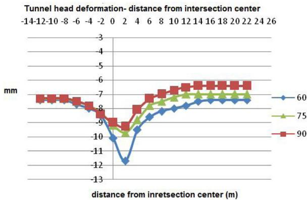
Figure 1. Variation of tunnel crest deformation with distance from intersection centre for different intersection angles
