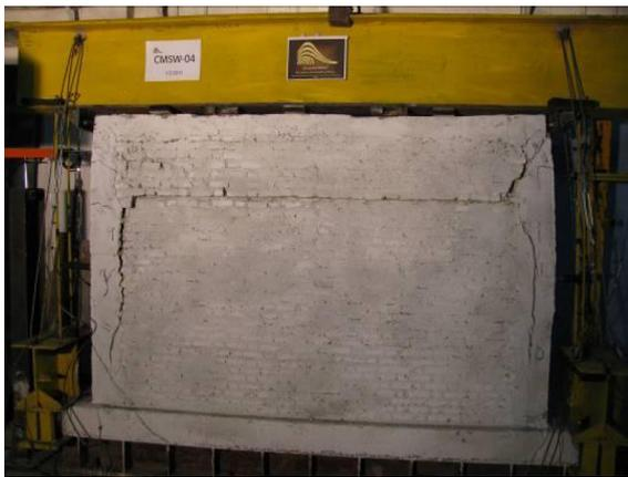
Figure 2. Cracks formed in specimen CMSW-04
