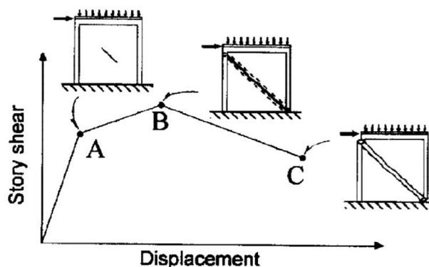
Figure 1. Typical curve from tests of confined masonry walls [6]
