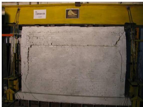
Figure 2. Cracks formed in specimen CMSW-04
