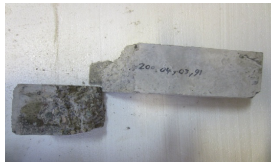
Figure 5. Failure surface of concrete beam strengthened with CFRP fabric in +80°C
