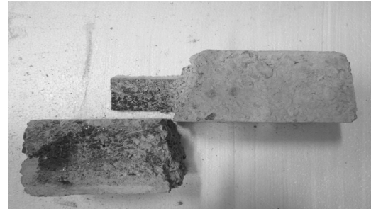
Figure 3. Failure surface of concrete beam strengthened with CFRP fabric in +20°C
