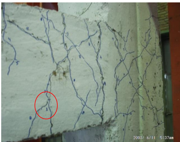
Fig.5-Location of first crack
